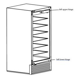
6. Rotate the door 180°, the door should installed the adjustable door shaft first, then relocate the door to the designed position.
