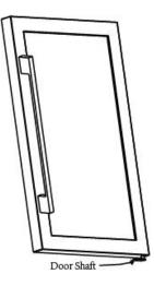
4. Unscrew the screws at the top hinge and lower hinge, and remove the the door hinge.Use a putty knife to prize up the screw hole cover which at the left side of the wine cellar, and re-cover the screw holes on the right side.
