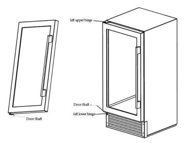
7. Adjust the door to make sure it is level with the top of the unit. Then tighten screws at the bottom.
